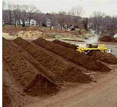
Photo: Windrow composting heaps
